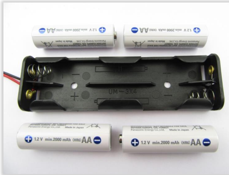
Figure 4 - correct polarity of rechargeables - hörbert with USB
