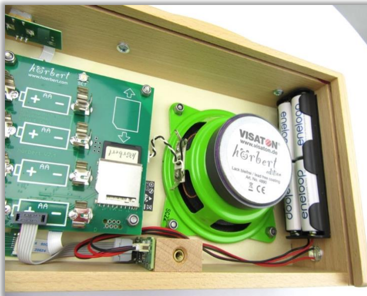
Figure 5 - Built-in power supply with accumulators
