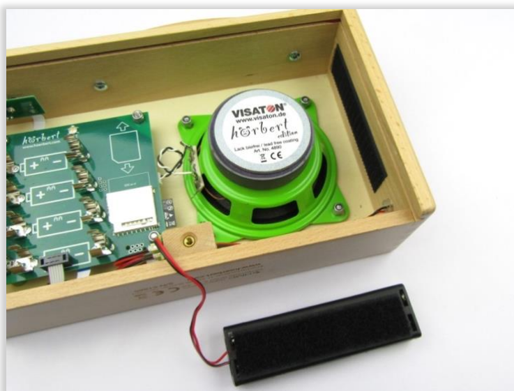
figure 3 - compartment for accumulators – Velcro Strip
